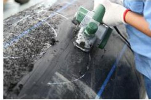
**\* We suggest scrapping the fusion zone by electric planer to remove the oxidized surface, this is very important.**
